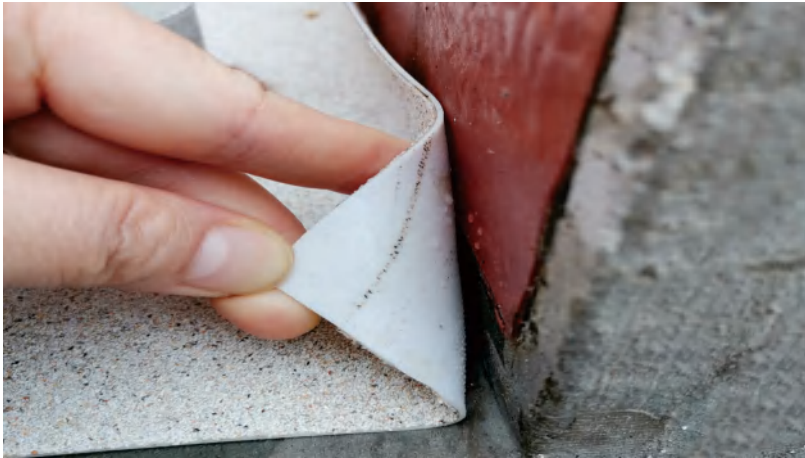
Smooth polymer sheets cannot bond with polyurethane.
