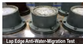
Lap Edge Anti-Water-Migration Test
