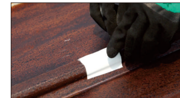
Nail Hole Reinforcement 钉眼加强
