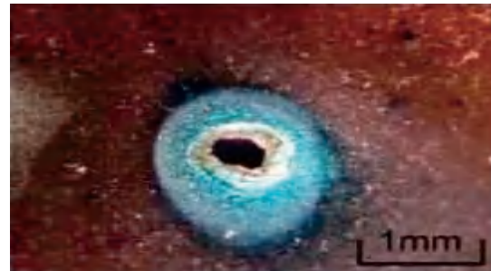
partialpitting has the greatest destructiveness and hidden danger, causing perforation
