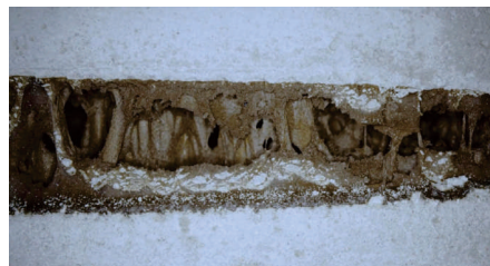
The CPS reactive adhesive firmly bonds to the concrete interface and can "grow" together with the concrete.
